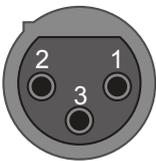
1-Shield pin    2-Hot pin    3-Cold pin
