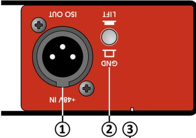
① **Signal output:** XLR terminal, isolated balanced output of the transformer, need to turn on +48V phantom power supply for PRO 148 proper working after connecting to the mixer.
